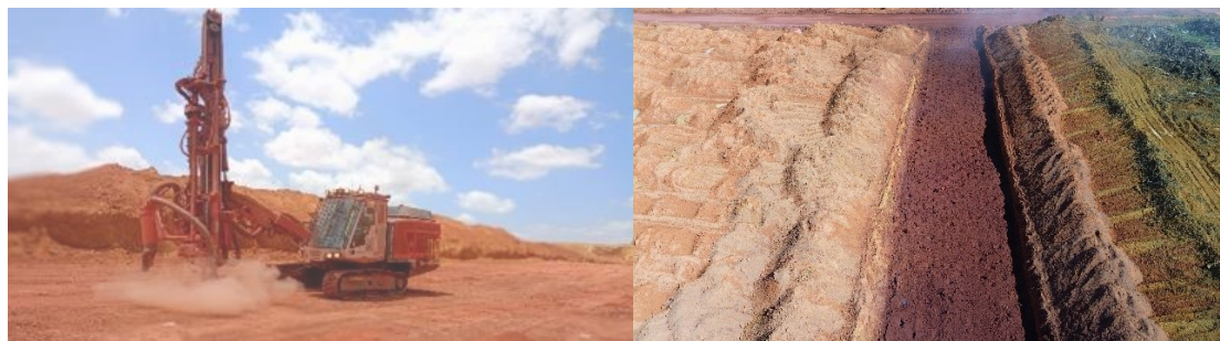
Figure 3. Micro-fragmentation. Left: Sandvik–DP1400i drill, Right: detonated area.
