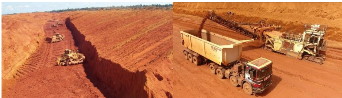
Figure 2. Mechanical fragmentation. Left: Dozer D11, Right: surface miner.
